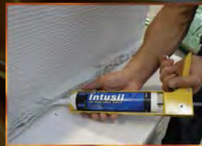
Sealing External Gaps On Our BAL-FZ Test Rig Prior To AS1530.8.2 Roof Test
